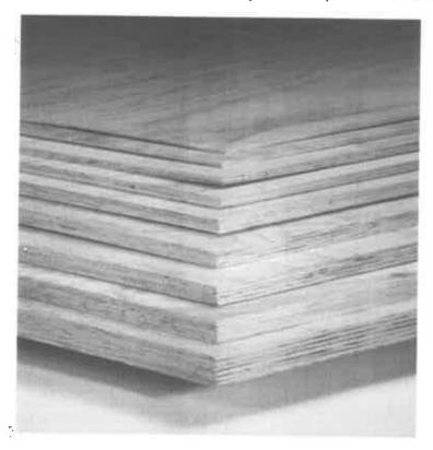
The outside plies are called face and back plies and the inner layers are called core layers. Typically a higher-quality, visually-appealing face is used on the surface of the board while the balance of the lower quality veneer makes up the core of the board. Usually the grain direction of the outer panel is in the direction of the longer dimension of the panel.
