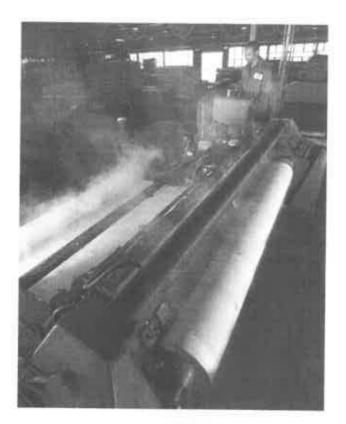
Logs are peeled using a rotary lathe into continuous rolls of wet veneer, 2.54m in width. These rolls are, in turn, trimmed using a clipper into veneer panels that are 1.28m in width.
