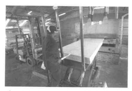
Boards are between 4mm and 32mm in thickness and are made to the standard dimensions of 2.44m by 1.22m (8 foot by 4 foot). Pressed boards are edge trimmed to size, inspected for defects, their faces sanded to provide a smooth and clean finished appearance if required and then strapped into pallets of approximately 2.7m³ or 1.5 tons. These are shipped in bulk to retailers who sell the plywood as individual boards.
