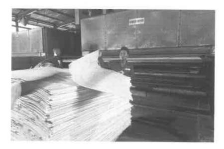
These are dried in **a** steam powered dryer for 10 to 15 minutes at approximately 150 degrees Centigrade to produce dry veneer with a moisture content of 6 to 10 percent moisture content.
