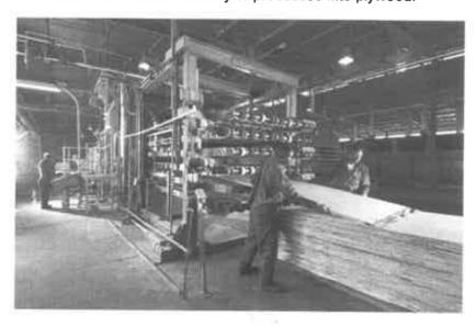
Plywood is processed by applying resin (urea formaldehyde or phenol formaldehyde) to alternate faces of the veneer and stacking this into packs. This pack is then inserted into a plywood press where it is compressed at high temperature and pressure to cure the resin and form the board.
