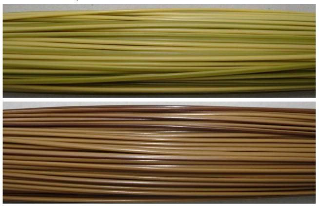
The samples were tested according to UL94 Standard Test procedures and Requirements UL94HB in five fold, the results are averaged values... Please note that the physical dimensions are only between 2 and 2.6 mm in diameter, which is not according to specification. The results are tabulated below.
